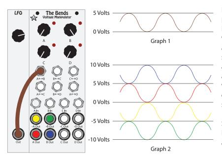
For a visual example, say you patched an LFO to the  $A \leftrightarrow B$  CV input, and that LFO was a sine wave, shown in graph 1. With the A and B knobs set to the positions shown (0V and 10V, since no inputs are patched), the CV-controlled averaging of those channels' values would result in four simultaneous outputs, shown in graph 2 (values shown are approximate).
